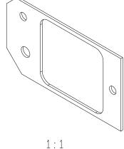
Material: Stainless steel Thickness: 1mm
